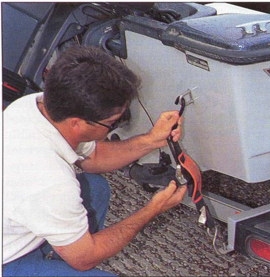
Transom tiedowns are necessary to prevent the boat from bouncing during towing.
